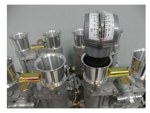
1. Close all 8 throttle air bypasses by fully inserting the idle adjust screws (green arrows).
