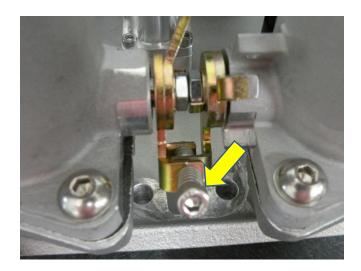
3. Check bank to bank synchronization and adjust hex linkage rods to ensure both banks open together.
