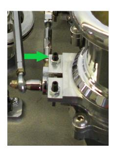
Adjust each turnbuckle rod (yellow arrows) to synchronize air flow through *the closed throttles*, on that bank. All eight throttles should be within 1 graduation on an STE air flow meter.
