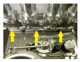
If necessary, adjust the hex linkage rods (blue arrows) to ensure both banks are synchronized.
