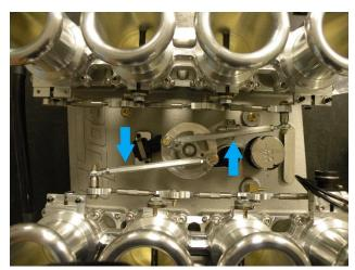
Lastly, tighten the throttle stop set screw on each bank until it makes contact with the tab on the shaft lever, then apply another ½ turn.
